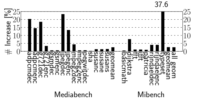
Figure 14: Dynamic instruction count increase due to ReplayCache compiler code generation; lower is better.
